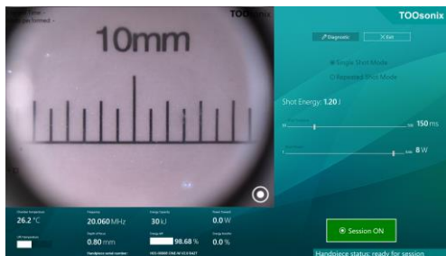
The TOOsonix Software with real-time optical video feed of the area being sonicated.
